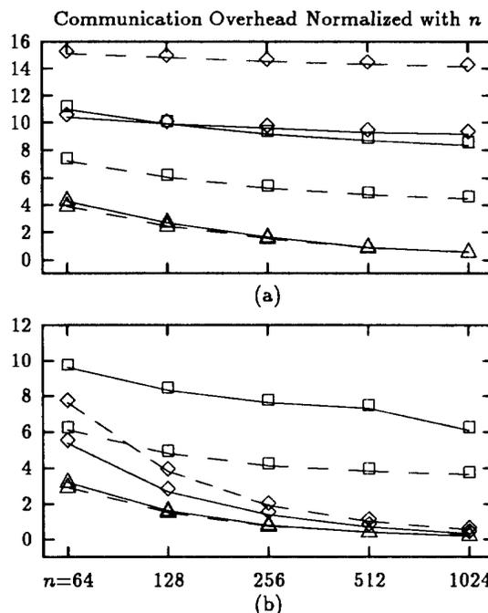
Figure 2. Communication overhead for wavelet decomposition (solid lines), and reconstruction (dashed lines);  $\square$ -BC2-MESH2/BC2-RMESH2,  $\diamond$ -DIST2-MESH2,  $\triangle$ -DIST2-RMESH2. (a) Taken to  $8 \times 8$  lowest resolution, (b) taken for only 3 levels. (Filter size is  $8 \times 8$ )
